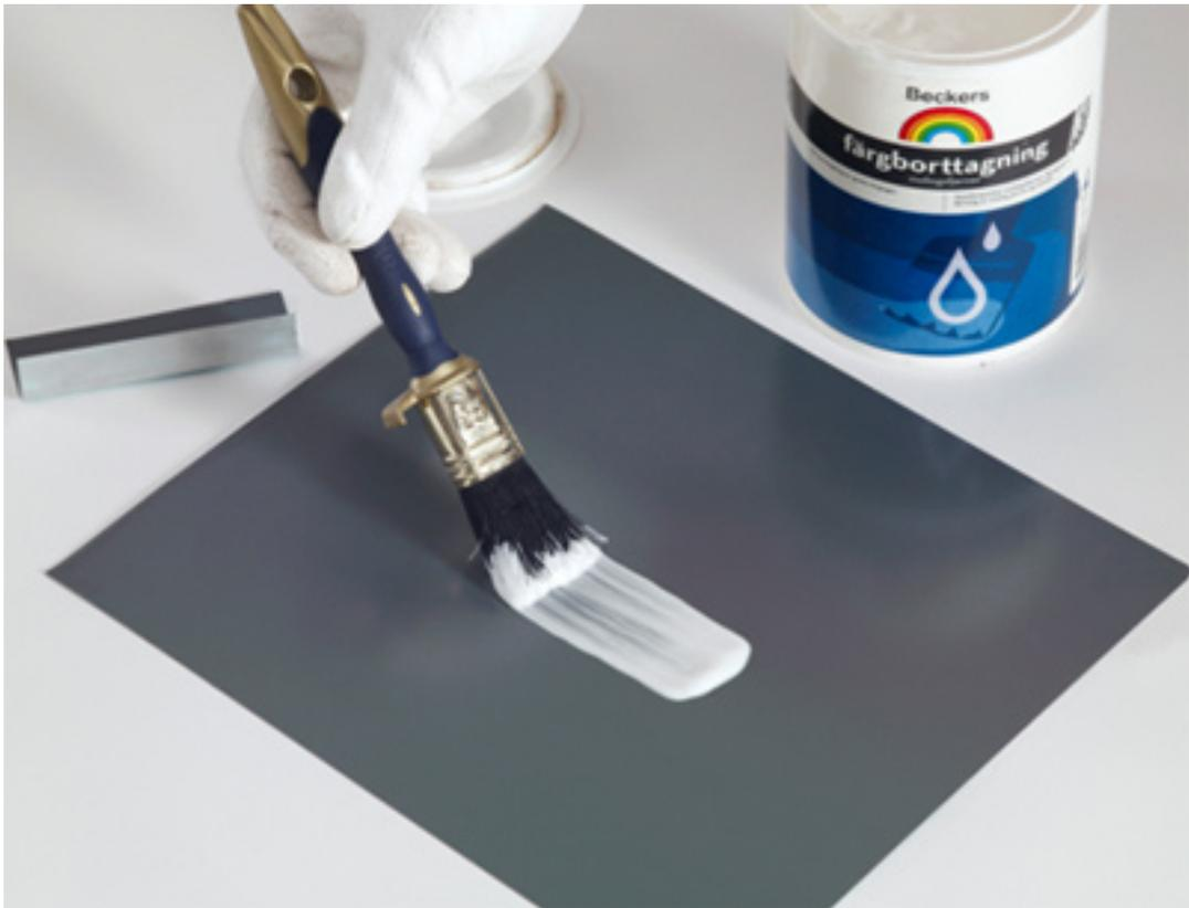
**Picture 3. Cover the surface with a Paint Remover**
